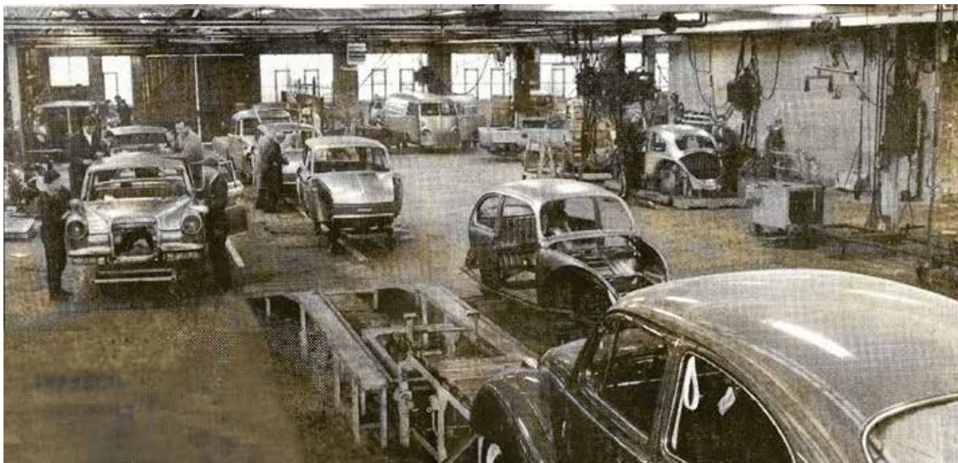
Volkswagen assembly on the Naas Road plant, Dublin ... The Beetle welding jig – the first to leave Germany – can be seen at top far right; in the foreground is the end of the Beetle finishing line; VW 1600 Variants and Transporters, as well as Mercedes-Benz 200 Saloons are also to be seen under assembly. Photo: GA Duncan/SBP
