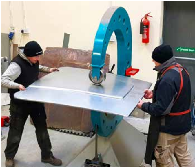
Pictured is the Jensen FF before restoration; the new bonnet being shaped on the English Wheel; and finally, the Jensen in glorious restored condition.
