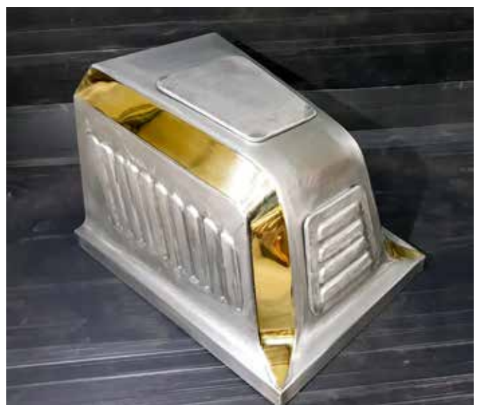
This 1902 Peugeot 'coal scuttle' bonnet was designed and fabricated by Tyrrell Coachworks using traditional methods, including a flypress and soldering irons. Although small in size, the bonnet construction is incredibly detailed, having 24 individual louvres and a brass inlay.
