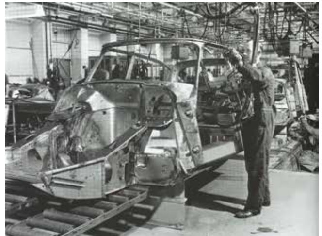
The revolutionary DS, being welded in Citroën's Slough factory in Berkshire, England. Photo: Citroën UK
