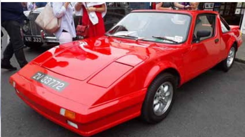
The Irish Clan Crusader, built in Newtownards, Co Down by Peter McCandless and based on the fiberglass-bodied Clan designed and manufactured by ex-Lotus engineers in England. In all, some 435 Clans were produced in the '70s, powered by an 875cc Climax engine.
