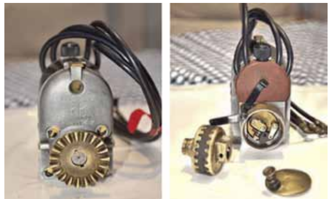
Front and rear view of the Rousseau Bignon (RB) magneto. The little window at the top at the front is to facilitate timing of the unit to TDC on No.1 cylinder. A lead from the cover plate at the rear is used to earth the Low Tension circuit and thereby stops the engine.
