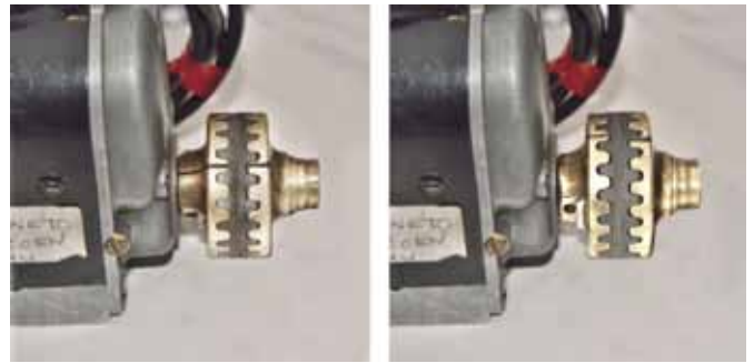
The clever 'Simms Vernier Magneto Coupling', The coupling is designed to make the magneto timing easy, with very fine advance/retard adjustment possible. Behind the toothed flange is an arrow that shows the operation of the magneto to be clockwise.
