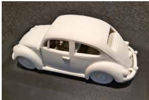
A VW Beetle printed with powder material
