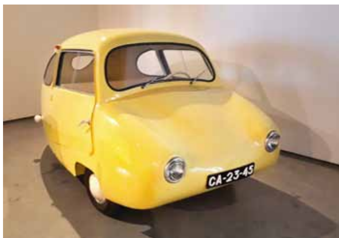
Nicknamed 'The Egg', with a single-cylinder 200cc air-cooled engine, the 3-wheeled Fuldamobil was built in Germany (in the town of Fulda) during the '50s. A 1955 Fuldamobil (Reg No. NRI 443) was owned by Paraic Pyne in Dublin and was in daily use until 1959.
