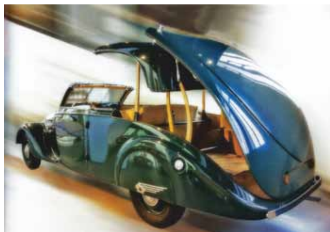
The Peugeot 'Eclipse' of 1937. The foldable roof system was designed by a dentist. It was another 60 years before the same feature was offered by car manufacturers. Buried during WWII, the car was recovered and restored by the museum - apparently with great difficulty.
