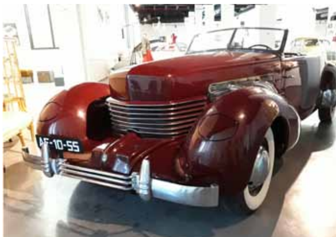
The compressor-supercharged sports version of the 8-cylinder, 4.7-litre American Cord. Part of the Errett Lobban Cord empire, which included Auburn and Duesenberg, this car was the creation of Gordon Buehrig, one of the most talented designers of all time.
