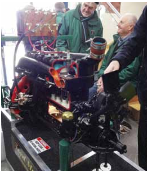
The cut-away Model T engine and transmission created by John O'Neill
