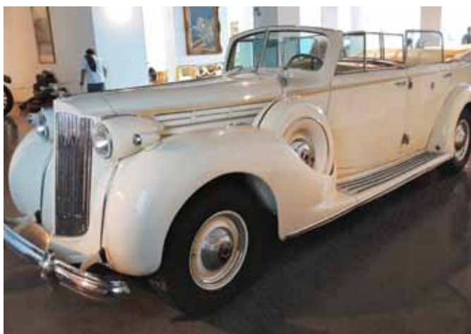
This 1939 Packard, is known as 'The White House Car' because it was the official transport of U.S. President Franklin Delano Roosevelt during his term of office. Powered by a V12, 175hp 7,800cc engine, it comes equipped with a cocktail cabinet.
