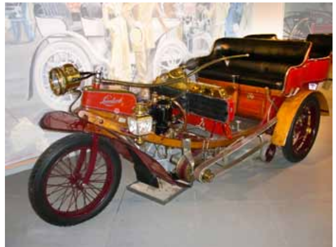
Lacroix et Delaville ‘La Nef’. Rear-wheel belt drive by a single-cylinder DeDion-Bouton engine
