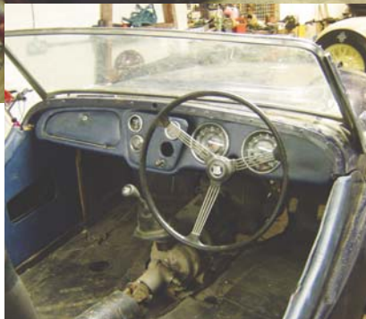
Below left: Inner sill fitted and A & B post repaired floor pan installed.
